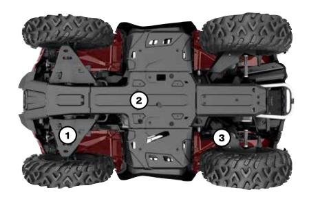
Our Plastic Plates glide smoothly and silently over obstacles, offering great protection in rough terrain. Made of ¼" (6 mm) thick abrasion-resistant thermoformed High Molecular Weight Polyethylene (HMWPE).
